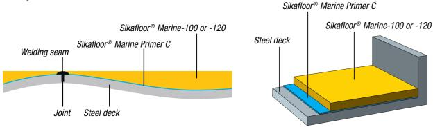
In addition to finish other Sikafloor®-systems, the Sikafloor® Marine-100 and Sikafloor® Marine-120 (after priming with Sikafloor® Marine Primer C) can be applied on top of existing hard foundations such as concretes and steel.
