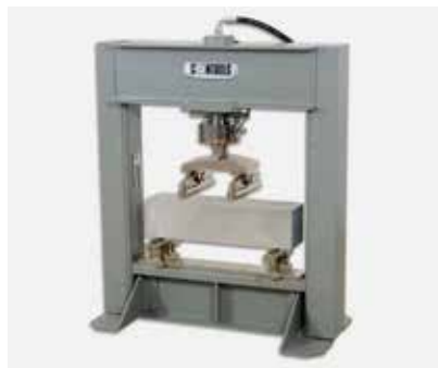
Beamtest: ASTM C1609
