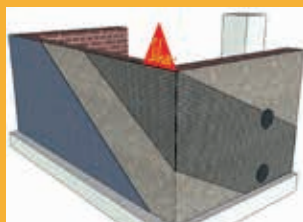
TECHNICAL ARTICLE Seismic retrofitting of masonry walls
