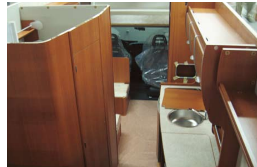
Bonded and sealed interior of a motorhome
