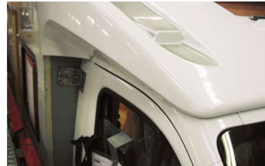
Bonded roof of a semi-integrated motorhome
