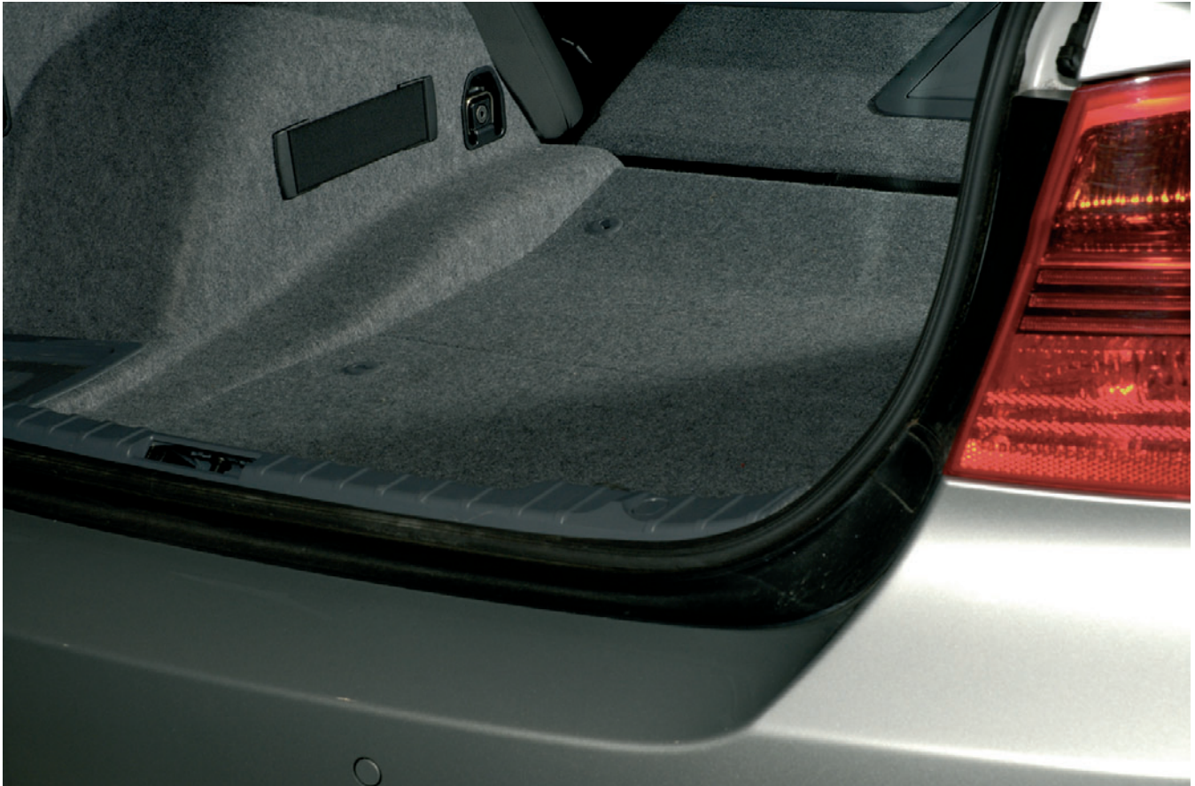
SikaMelt® technology used in the bonding of load floors
