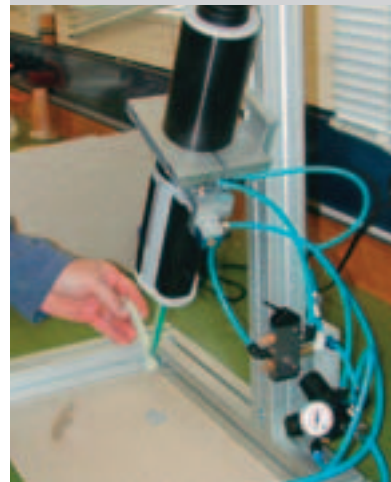
The fixed installation of a foot controlled pneumatic cartridge gun simplifies the bonding of small parts
