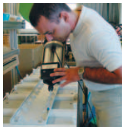
Bonding of a GSM antenna cover to the base with a standard refillable gun suitable for SikaFast®
