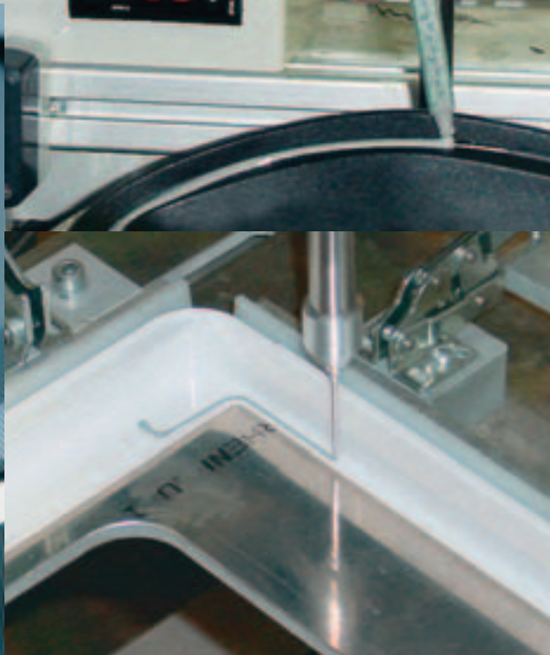
Robot application of SikaFast® adhesive systems allows for shorter production cycles as required in the manufacture of furniture
