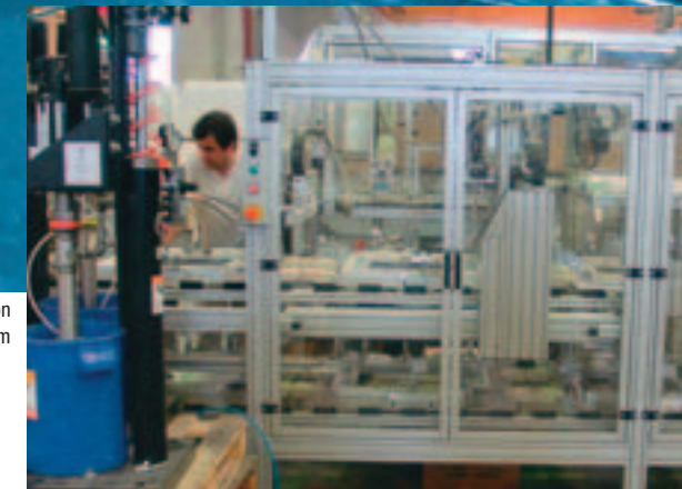
Integration of SikaFast® in an automated production line using a pumping and dosing system
