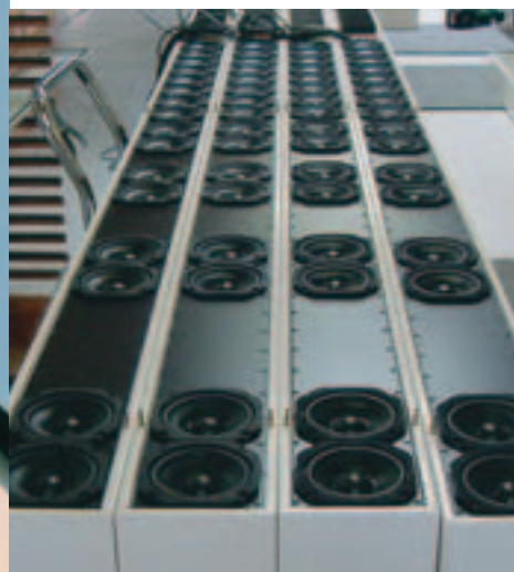
Efficient production of loudspeaker cabinets by bonding the front panels into the metal box eliminating mechanical fastening, offering a smooth appearance
